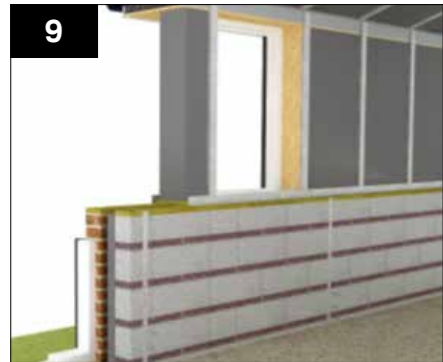
Wall straps to be positioned 300mm from host wall / internal corners, then fixed at no more than 1500mm centres.
