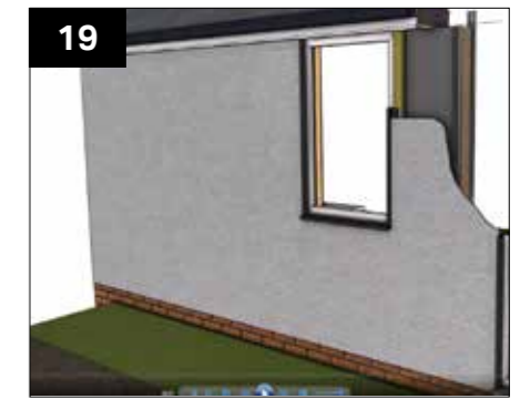
In the case where the new wall is within 1 metre of a boundary Calcium Silicate Board will be provided. This needs to be installed before battening if a cladding is being used.
