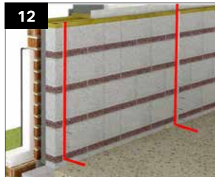
Please note where the wall is less than 600mm in height the end of the strap should be bent at 90deg and fixed to the slab). Existing floors need to be considered if staying in place for example tiled floors.
