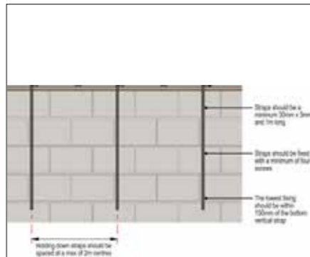
Fixed with a minimum of four hardened nails 4mm in diameter *75mm long, or No12 wood screws *50mm long into plugs (where fixed to masonry). Min 4 fixings required and with the lowest fixing secured within 150mm of the bottom of the vertical strap.
