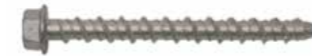
Base tray to foundation example fixing: M6 x 85mm Concrete Bolt with a minimum 1kN pull out. Fixing choice is dependent on substrate.
