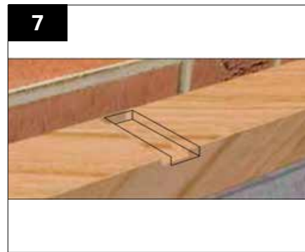
The timber is to be bedded on mortar and strapped down to the internal face of the wall. The timber is to be rebated/notched so that the wall strap sits flush into the timber. Approx. 95x44mm treated timber to be used
